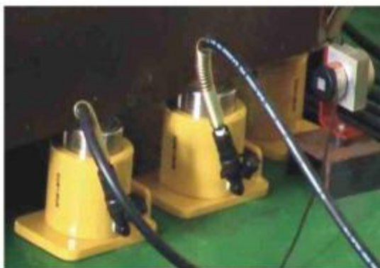
RSCS-502 捷運系統同步實例應用 RSCS-502 Rapid transit system Synchronous Lift application
